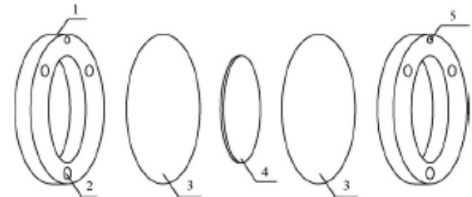
The schematic diagram of the POCIS device (1) PTEE holder, (2) screw, (3) membrane, (4) sorbent and (5) hole.
