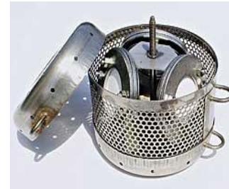
The schematic diagram of the POCIS device (1) PTEE holder, (2) screw, (3) membrane, (4) sorbent and (5) hole.
