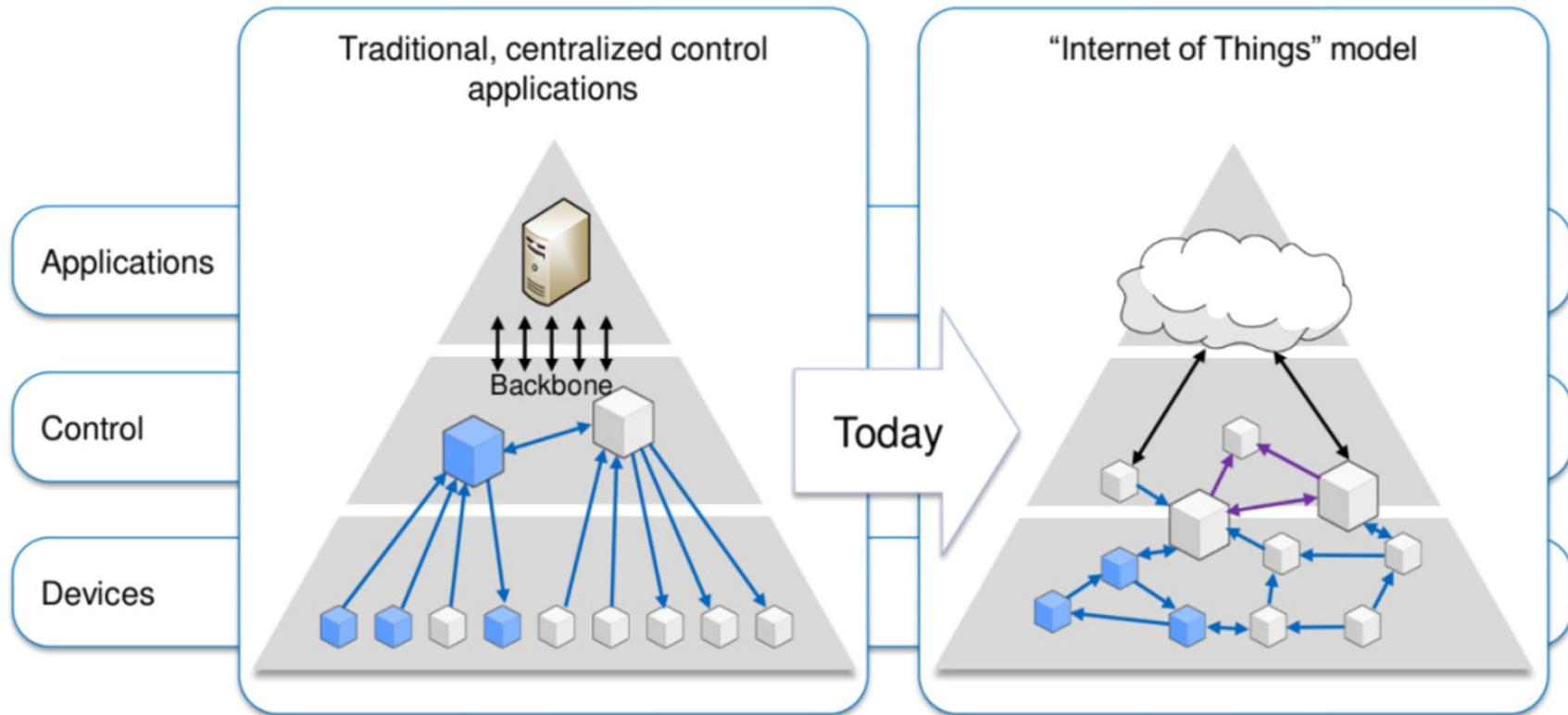
IoT: decentralized interconnected field devices : additional sensors can „easily“ be added
