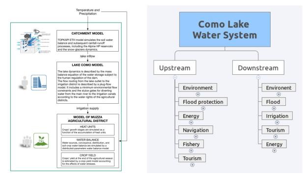
Figure 2. The Lake Como water system sectors and integrated model
