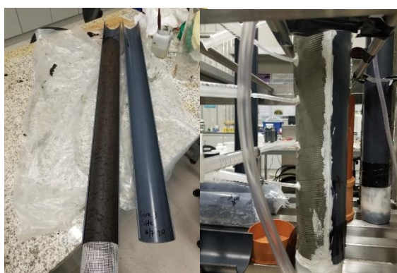
Figure 4: Beginning (left) and end (right) instrumentation of soil samples in NUIG laboratory.
