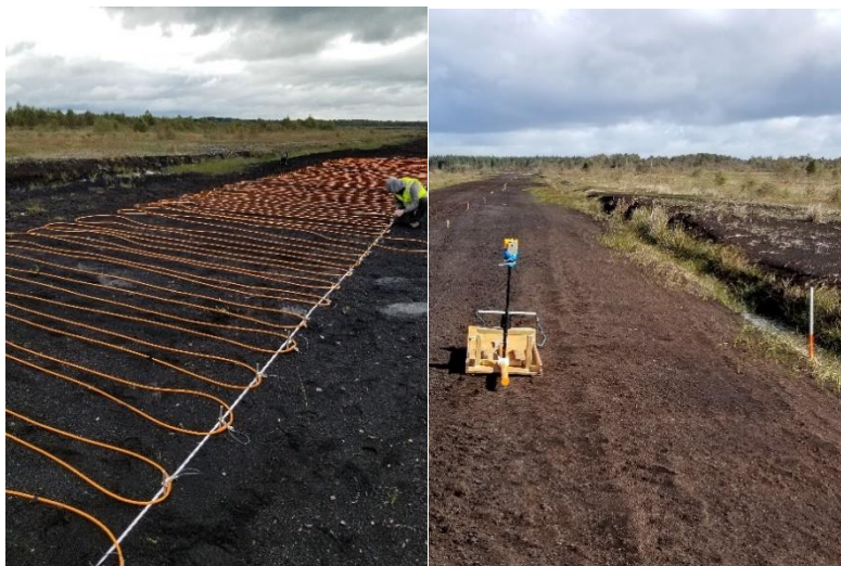
Figure 2: ERT survey line (left) and EMI survey instrument and reach (right)
