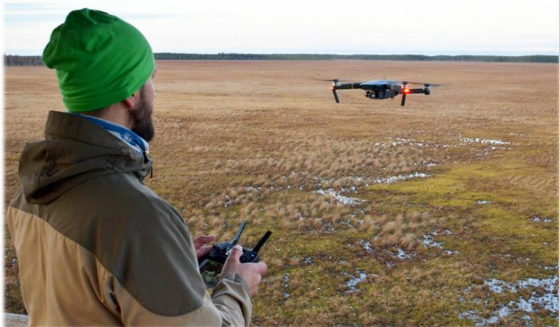
UOULU researcher Lauri Ikkala (Olvassuo, Finland). Peatland restoration sites are studied with drone imaging and mapped with near-infrared and thermal infrared wavelengths to produce orthomosaic images, digital elevation models and a variety of moisture and vegetation indices.
