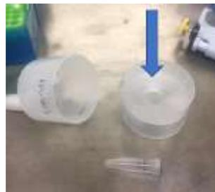
Figure 4: Collection cup with filtered sample
