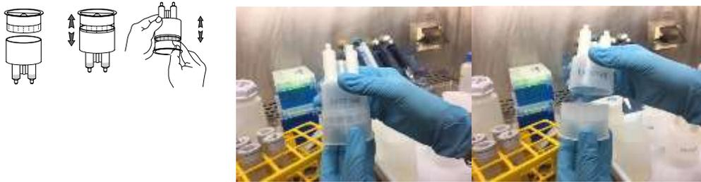
Figure 3: Schematic procedure to proceed with the recovery of the concentrate
