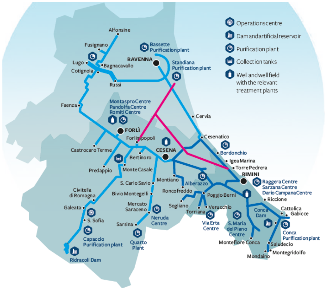
Figure 2. “Acquedotto della Romagna” (Romagna Aqueduct) water network, which link the Ridracoli reservoir to the majority of the municipalities in the Romagna region.
