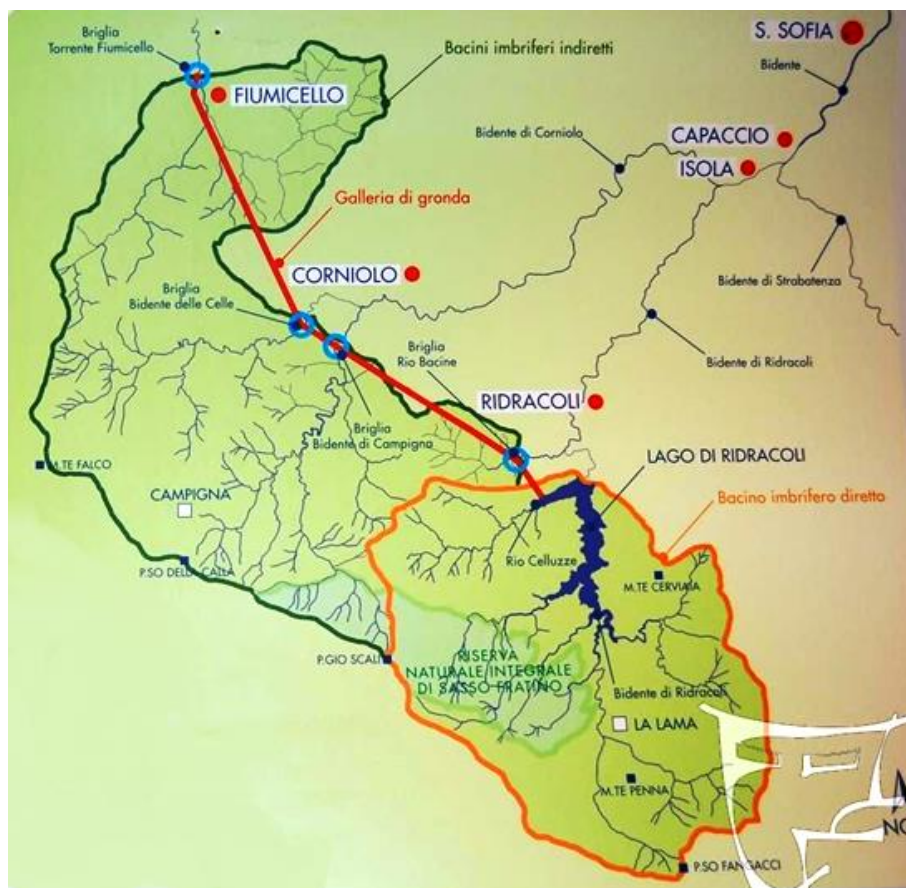
Figure 3. Ridracoli reservoir system: orange contour refers to the hydrographic basin closed at the dam, blue circles to the weirs in the diversion watersheds and red line to the underground channel.
