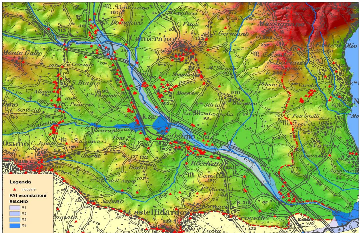
Fig. 4 DTM cartography with flood risk areas and civil or industrial buildings in red.
