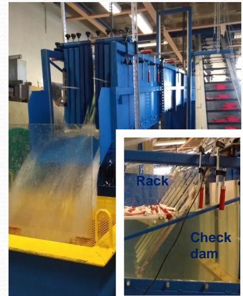
Slit check dam, and of the rack from the transparent side-wall
