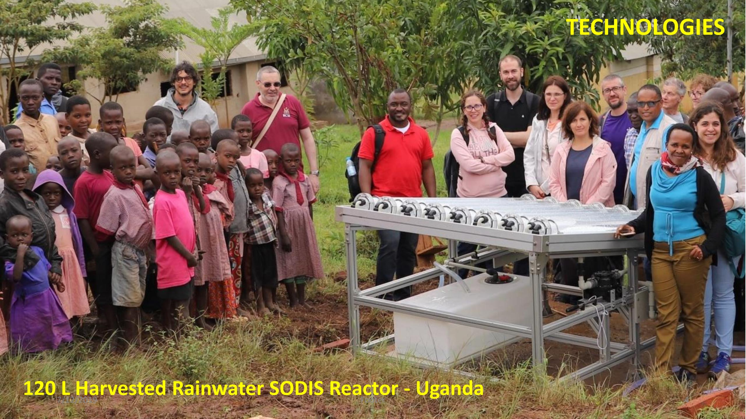
120 L Harvested Rainwater SODIS Reactor - Uganda
