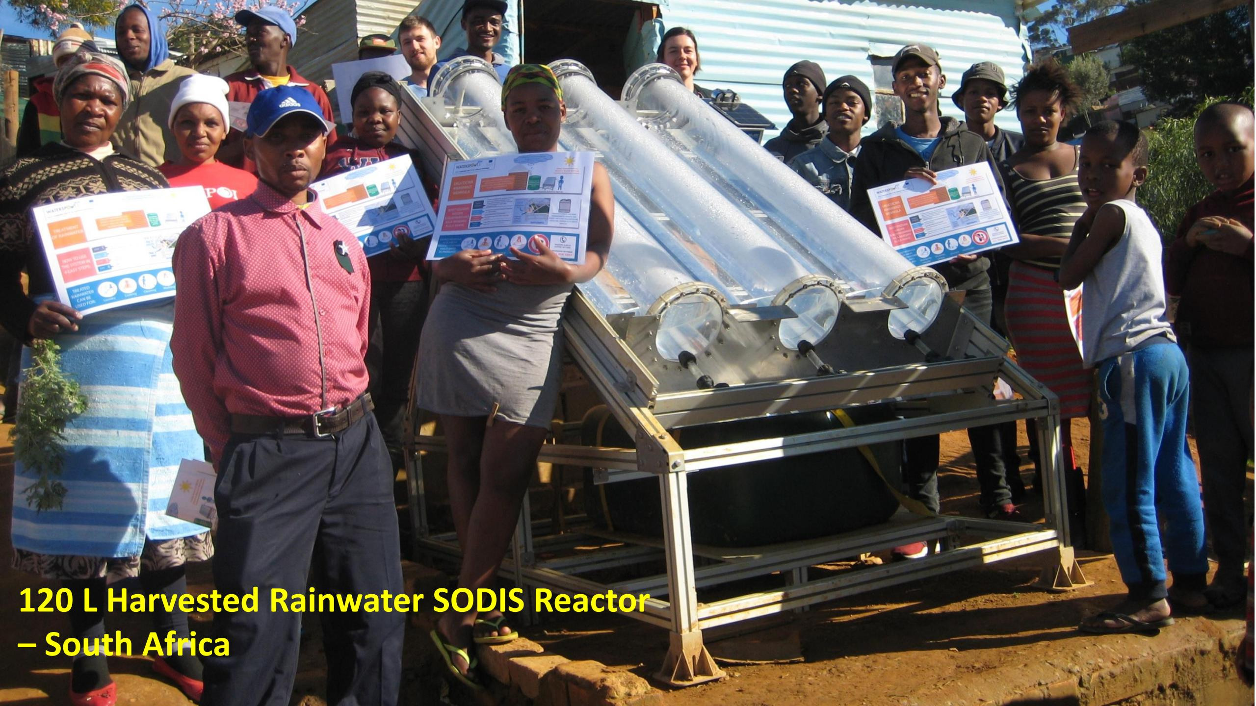
120 L Harvested Rainwater SODIS Reactor
